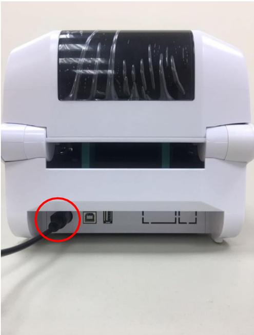
Step 2: Using the USB Type A <-> Type B transmission line, connect the Type A terminal to the computer, and connect the Type B terminal to the machine
