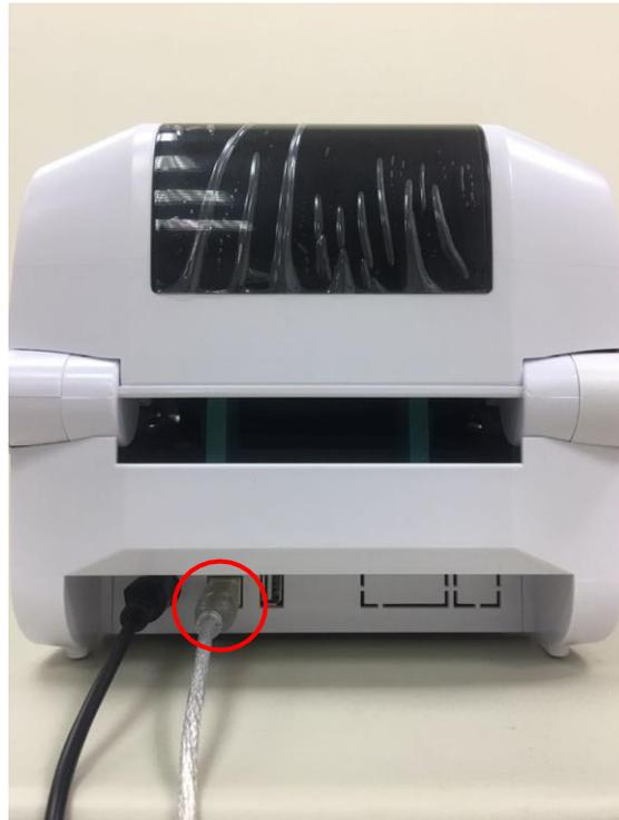
Step 3: Insert the desired USB HID device (Barcode Scanner in example) into the USB Host port of the machine.
