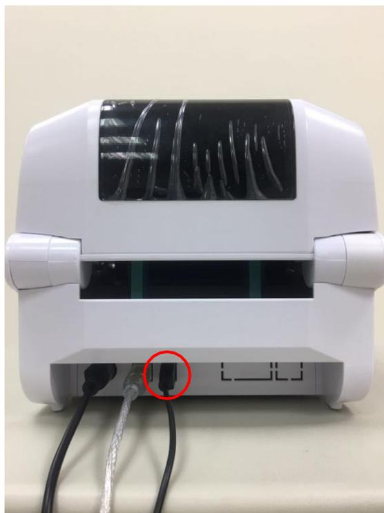
Step 4: Start the machine power switch (press the number "-").
