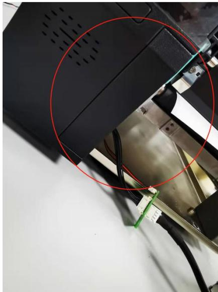
13. Card the small cutter bump into the corresponding groove in the figure below:
