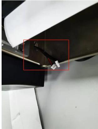
**10.** Insert the Black Red Line End and the Black Line End into the adapter plate Number 1 and Number 2 line ports in the figure below:
