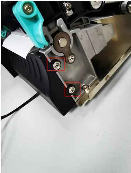
2. Remove the sensor and baffle screws.
