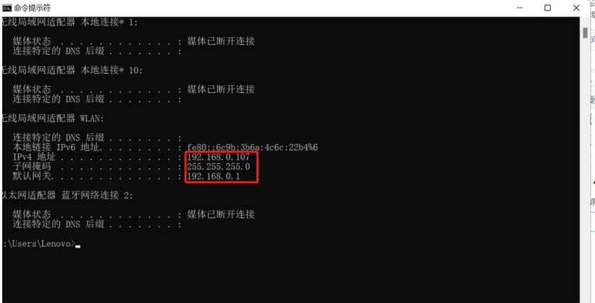
5. The IP address, gateway address, and subnet mask in the PrinterUtility must be consistent with the desired WiFi connection. **Note: (The IP address does not conflict with other connected devices)**
