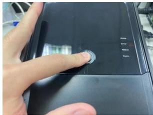
1. To confirm the paper and ribbon are properly installed in the printer and start the printer.
