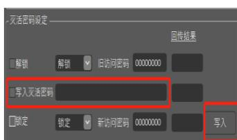
It can be set in the Kill Password Setup area of PrinterUtility RFID Test plate ([detailed explanation of the plate can be referred to in Section 8 of Chapter 5](#)). Enter the Access password to be written in the input box of Access Pwd., then click the "Write" button on the lower right corner. [Refer to Appendix A for details of returned error code.](#)
