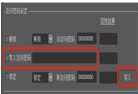
Click the "Access Password Setup" in PrinterUtility RFID Test plate for setting ([Detailed explanation of the plate can be seen in Section 8 of Chapter 5](#)), enter the access password to be written in the input box of "Access Pwd.", and then click the "Write" button, [return error code details can be seen in Appendix A.](#)
