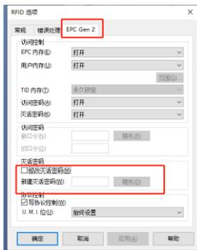
Open BarTender and add the RFID tag ([the details are described in Chapter 6, Section 5](#)). After adding the RFID tag, open the RFID option ([details are described in Chapter 6, Section 6](#)). In EPC Gen 2, check the button to change the Kill password and enter the Kill password in the password box. Click "Apply" or "OK" below. After the Kill command is executed, labels die permanently and cannot be used any more. Labels that are not configured with the Kill Password cannot be killed.
