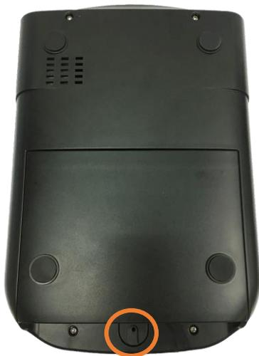
5. Turn the printer upside down, remove a screw located on the bottom cover, and open the bottom cover.
