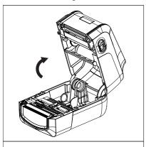
1. Press two buttons on printer two sides to lift and open the cover.
